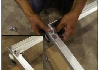
Slide the bolt of the casters (L) through the holes of (A) and (B). Secure the casters to the frame using the 1/2" nuts and 1/2" lock washers (H).
