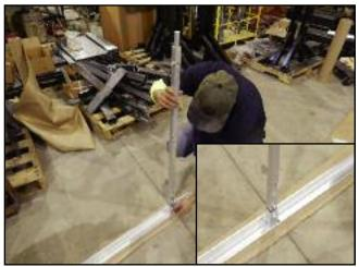
Lay out the (2) 48" angled bottom bases (A) so that the pre-drilled holes are on the floor, and insert the 40" square uprights w/round bar (C) into (A) so that the round bar is facing up as shown in the picture above. (NOTE: The pre-drilled holes on (C) are numbered. Have the numbered side facing outward.)
