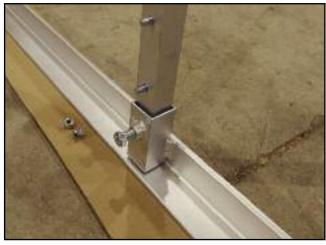
Once (C) is inserted in to (A) tighten the bolt to secure the upright. Do this to both sides.
