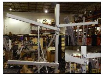
Attach (20) 18" square tubing (G) to both uprights (C) and (D). Secure (G) in place using the 2-1/2" bolts (J) and 1/4" lock nuts (K). The pre-drilled holes on (G), (C) and (D) are numbered for easy placement. Please see next picture (#8) for example of the numbering.
