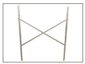
The above picture shows how the flat bar braces (F) should look once they are attached to (C) and (D).
